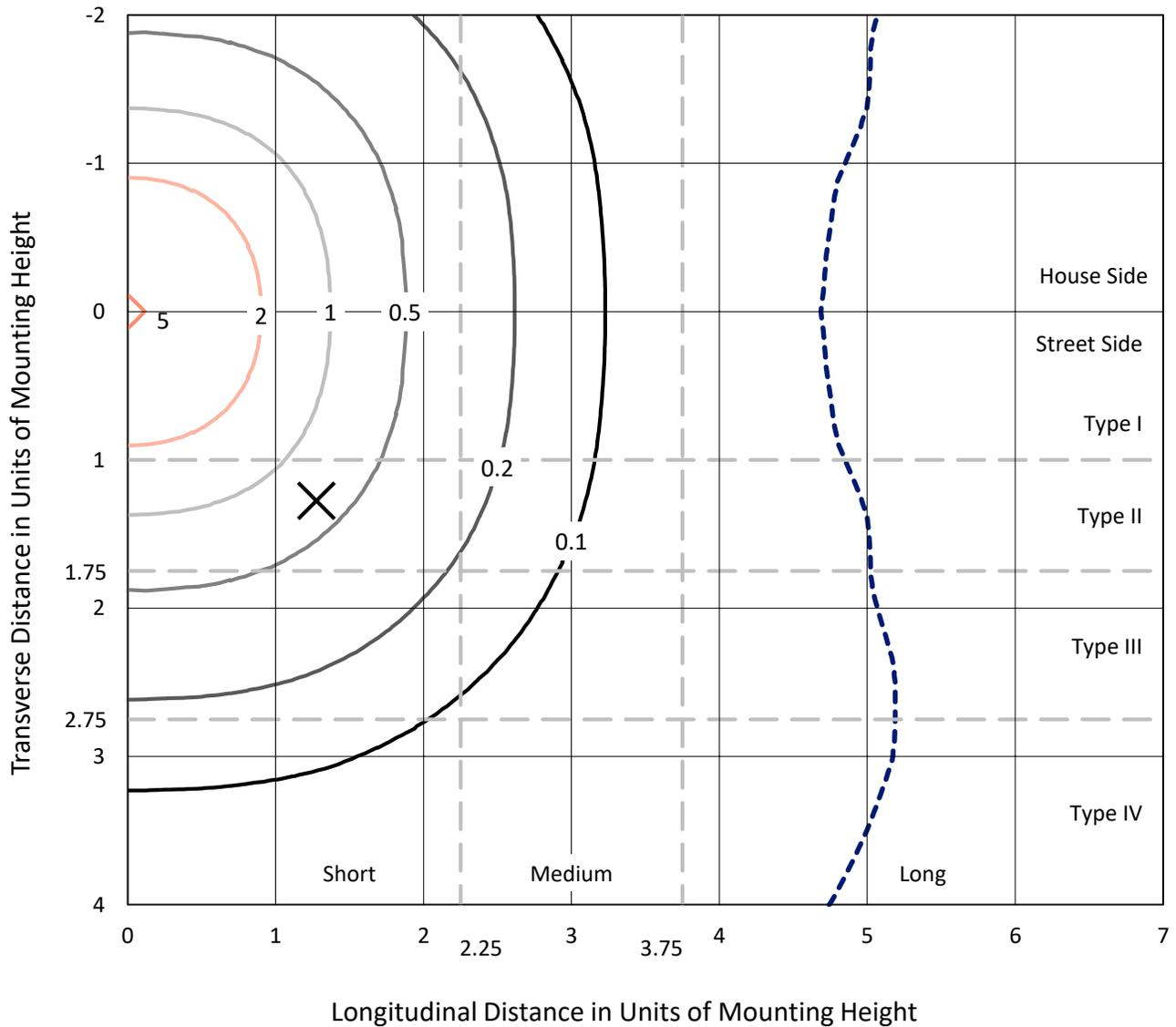
Based on 20 foot mounting height. Maximum calculated value = 5.1 fc
